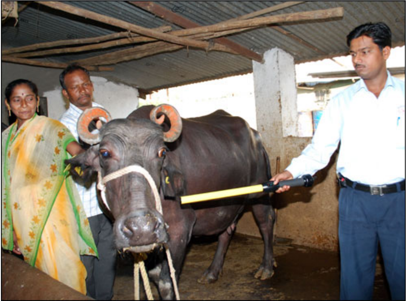
A Chitale service provider uses an Allflex handheld interrogator to read a water buffalo's ear tag.
